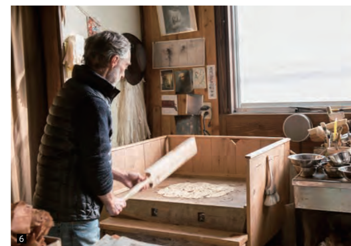
⑤ The chiritori step, which determines the quality of washi . Impurities, such as the black skin sticking to the paper material, and discolored parts are carefully removed in cold running water; ⑥ The koukai step in which the fibers are softened using a wooden stick. This tool was also hand made by Rogier. ⑦ Paper made from the fibers is mixed with water and sunset hibiscus sap. ⑧ Washi is dried in the sun. The paper is finished when it is fully dry.
