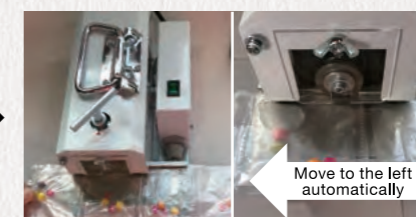
⑤ Carefully bring it into contact with the end of the rail. When the part to be bound is sandwiched between the teeth, the layer of doses will automatically move to the left.
