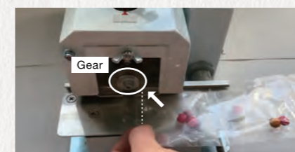
④ Slide the layer of doses to the position at which the top dose comes into contact with the teeth.
