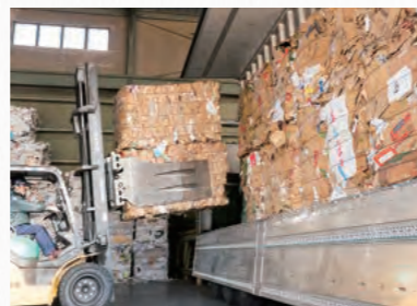
Vinyl strings and other unnecessary objects are manually removed from the collected waste paper. Then, the waste paper is put into a machine called baler and compressed into an about one-ton mass before being bound with annealed wire and shipped to paper manufacturers.
