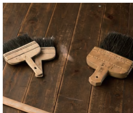
Uchibake (right) is designed to mix the fibers of the top and bottom washi, whereas nadebake (left) is used to apply wheat gluten glue to the washi.
