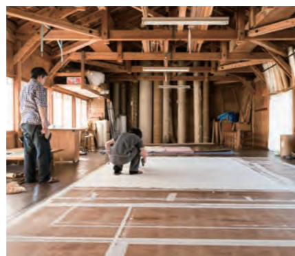
The spacious atelier is dedicated to yuton making. The work of pasting washi must continue ceaselessly in order to prevent the glue from drying.
