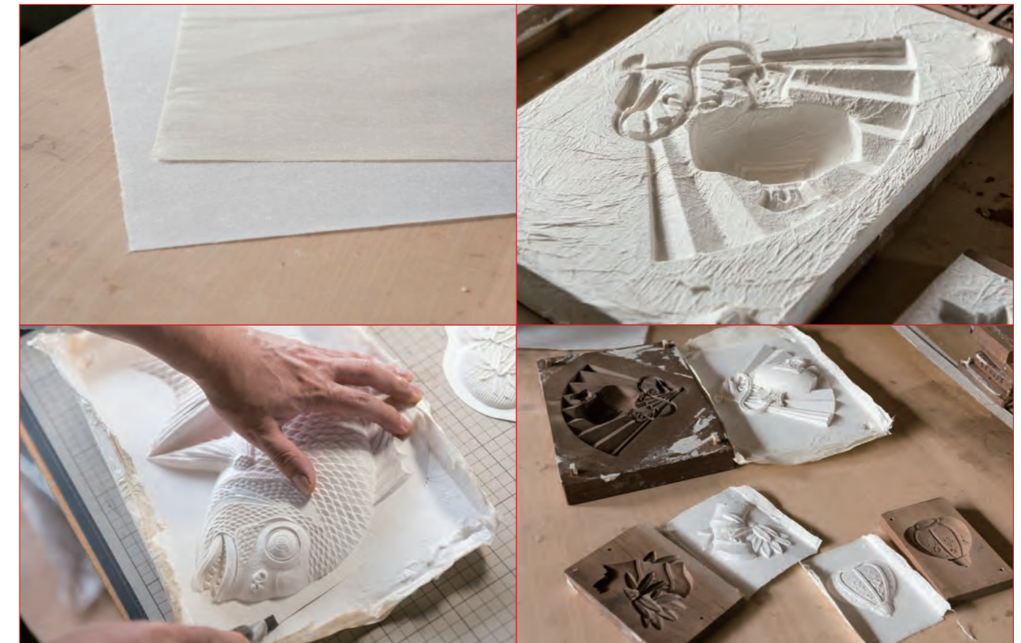
(Upper left picture) Nishinouchi-gami. Sarashi is white because it is bleached in the sun. Misarashi is brown because the fibers of kozo remain. (Upper right) A confectionery pattern and washi are glued together using a brush and shade-dried for half a day to one full day. (Lower left) Sticking roughly cut blank spaces together and shaping them into a single work. (Lower right) Single parts peeled off from the wooden pattern. Details of the wooden pattern are clearly transcribed.
