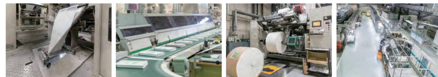
IWAOKA CORPORATION has patented technologies that have enabled the company to achieve four-color full-color printing on super-thin paper, 18g/m 2 , a first for Japan. It has now also successfully carried out test printing on paper with a thickness of just 14g/m 2 , making it as thin as tissue paper.
