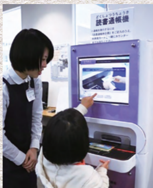
There are two types of reading passbook terminals that can print information in passbooks: an autonomous model (see photo) and a compact model. Photo taken at the Kudamatsu City Library.
