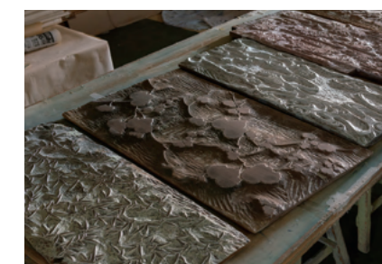
The production of large-sized paper (approximately 90cm x 180cm) led to the use of woodblocks larger than 90cm for making karakami paper in the Tokyo area.
