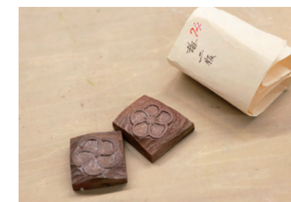
Small-sized woodblocks known as kiri-mochi (literally "cut rice cakes"). They can be arranged in various combinations to create diverse patterns.
