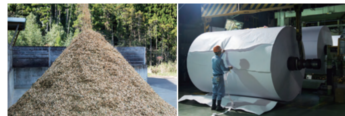
Felled bamboo stalks are collected and sent to the chip mill. Bamboo chips processed here are pulped in a digestion kettle called a batch boiler, and then go through the paper-making process to become Takegami paper.
