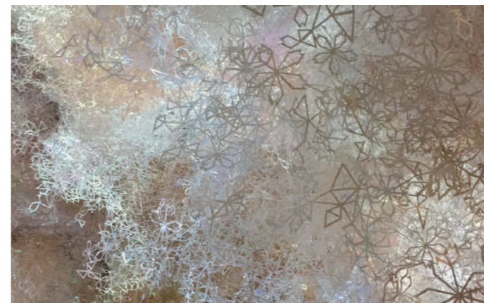
Decoration made with patterns of detailed, paper cutout-like cherry blossoms. Laser can precisely recreate digital data's minute expressions in a way that would not be possible with die-cutting.
