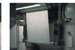
3. Printing Designs are applied with a gravure printing process employing intaglio printing. Water-based inks are used due to environmental and safety considerations.
