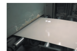
2. Coating After the base paper is coated with paste sol, a drying furnace and cooling roll are applied to create the foundation for the wallpaper.
