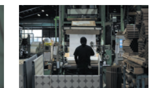
5. Inspecting & Packaging Stringent checks are conducted in each stage of the inspection process with inspectors and CCD sensors. Rolls are checked for differences in hue, left-right imbalances, and more.
