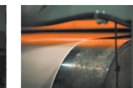
4. Foam Expansion & Embossing Printed mother rolls are made to expand in a foaming oven, then pressed with embossing rolls after being heated.
