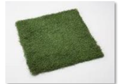
Artificial grass made of paper yarn
